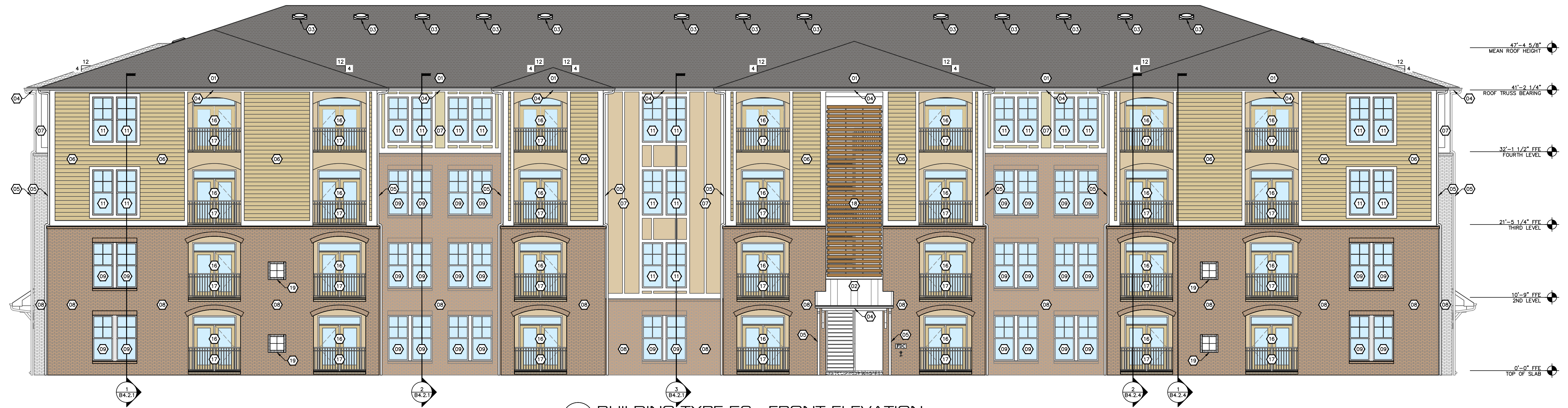
1 BUILDING TYPE 56 - FRONT ELEVATION 1/8" = 1'
